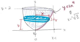
Each slice moves a different amount and each slice has a different amount of force acting on it (different volumes), so we need to do an integral.
