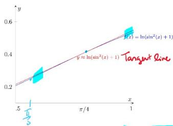
Close to the point of tengency, the values of the function can be approximated by the values of the tangent line
