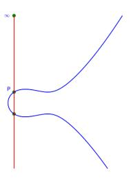
A line through *P* and  $\infty$  is vertical: the other intersection is the reflection through *x*-axis.
