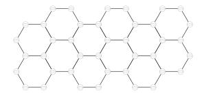
This is a single plane of graphite, called *graphene*. A piece of graphite consists of millions of these planes layered in a stack. The chemical bonds between the planes are much weaker than the bonds inside the planes, which explains why pencils write—the graphite can be sheared so that the planes slide off and are left on the paper.
