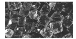
The explanation for the cubical external shape is the simplest one that we could imagine: the internal shape, the way the atoms lie, is also cubical. The internal structure is pictured below. Salt is sodium chloride, and the small spheres shown are sodium while the big ones are chloride. To simplify the view, it only shows the sodiums and chlorides on the front, top, and right.
