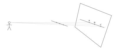
It is not a orthogonal projection since the line from the viewer to C is not orthogonal to the image plane.
