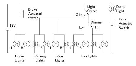
The designer of such a network needs to answer questions like: How much electricity flows when both the hi-beam headlights and the brake lights are on? We will use linear systems to analyze simple electrical networks.
