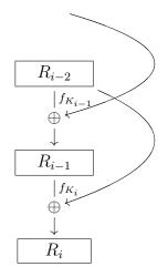
The final output of the Feistel cipher is the inverted pair  $R_rL_r = R_rR_{r-1}$ , which allows the Feistel cipher to be inverted by running through the same algorithm with the key sequence reversed.
