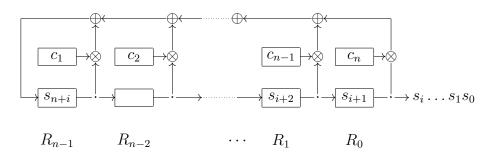
Before discussing the mathematical definition of linear feedback shift registers (LFSR's), we address the question "Why?". A LFSR is essentially an elementary algorithm for generating a keystream, which has the following desirable properties:
